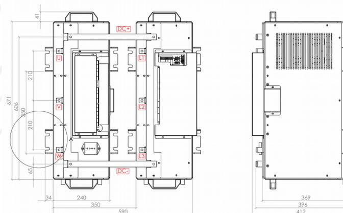
Active Front-End regenerative frequency converters make possible recover the energy to the electric network during braking or changing direction of motor.
