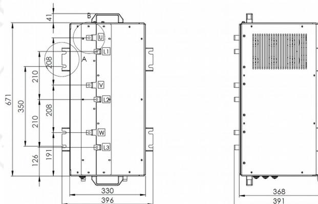
Example of mechanical view of the MFC810 315 kW 1.1kV Active Front-End (AFE) frequency converter.
