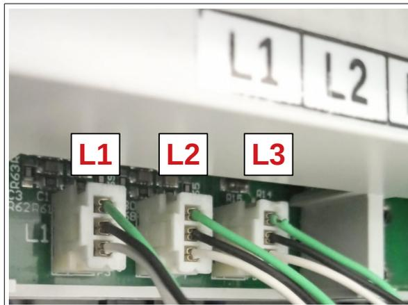
**Fig. 6.2.** Connecting PA3209NL transmitters to PS Energy Guard
