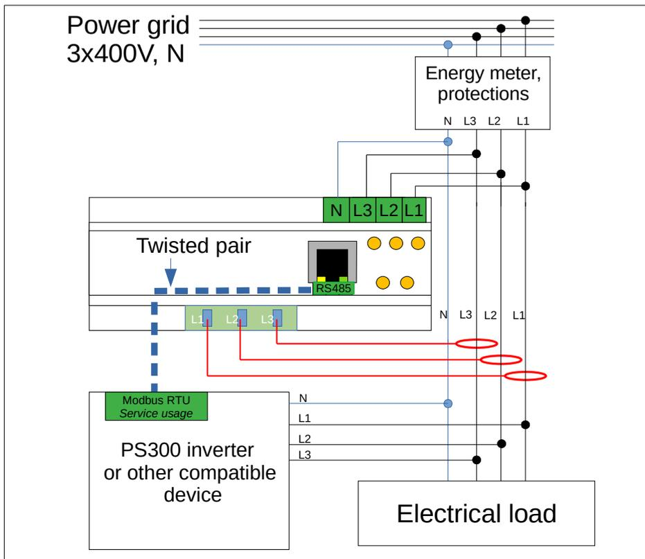
**Fig. 5.6.** PS Energy Guard 3F-Z - connection diagram
