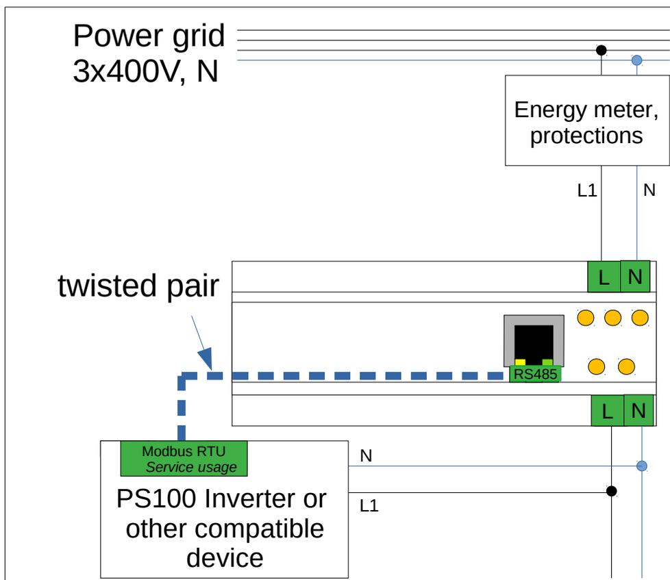
**Fig. 5.2.** PS Energy Guard 1F-W - connection diagram
