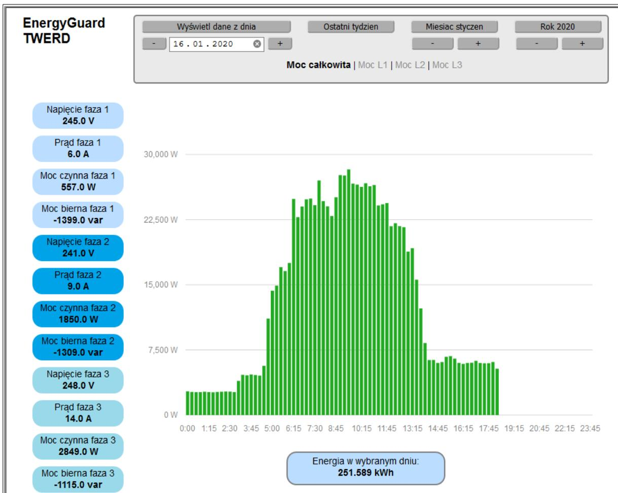
Fig. 9.1. Information panel preview for PS Energy Guard through [www.inverters.pl](http://www.inverters.pl)
