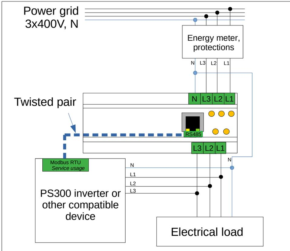
**Fig. 5.4.** PS Energy Guard 3F-W - connection diagram
