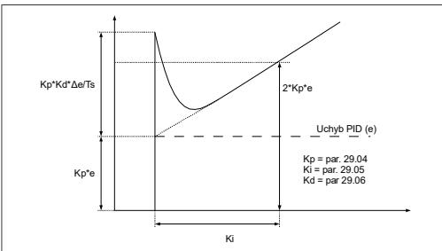
**Fig. 4.1.** Reaction of the PID1 controller to the error message in the open feedback loop
