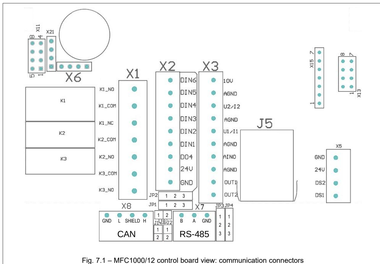
Fig. 7.1 – MFC1000/12 control board view: communication connectors
