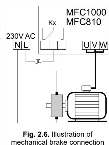
Fig. 2.6. Illustration of mechanical brake connection
