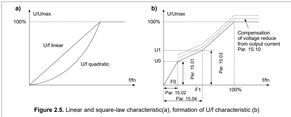
Figure 2.5. Linear and square-law characteristic(a), formation of U/f characteristic (b)
