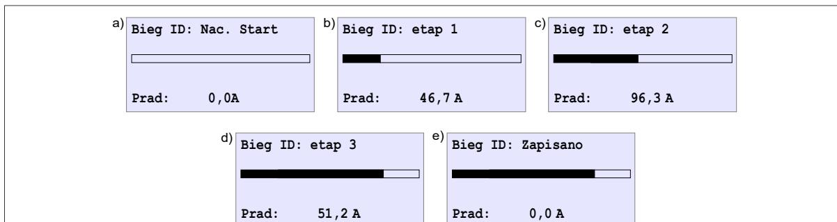
**Fig. 3.1.** The right course of the identification run (the current values during the run depend on the entered nominal data of the motor and the moment of the given stage)
