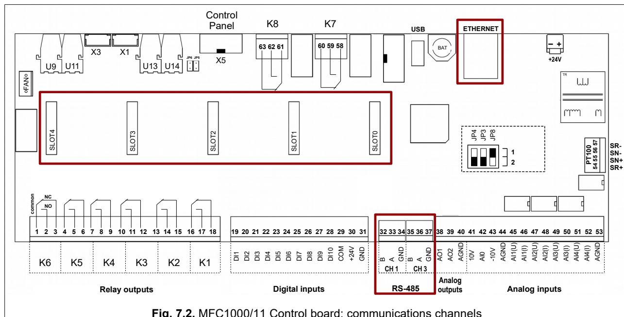
Fig. 7.2. MFC1000/11 Control board: communications channels
