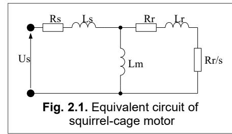
Fig. 2.1. Equivalent circuit of squirrel-cage motor
