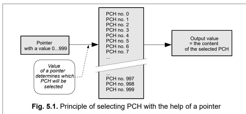
**Fig. 5.1.** Principle of selecting PCH with the help of a pointer
