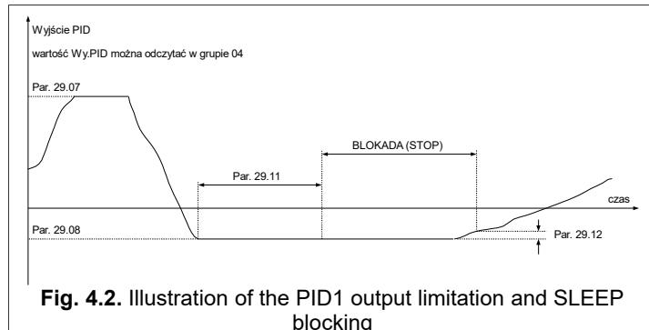
**Fig. 4.2.** Illustration of the PID1 output limitation and SLEEP blocking
