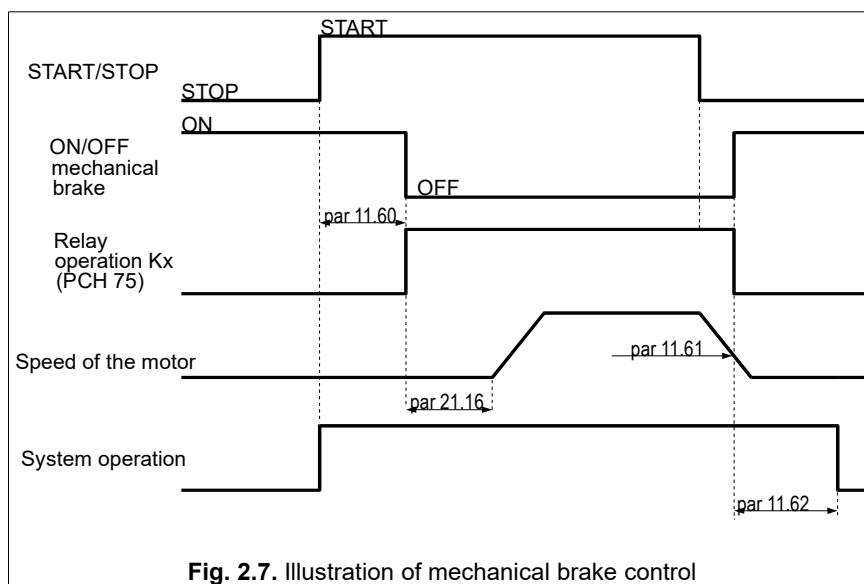
Fig. 2.7. Illustration of mechanical brake control
