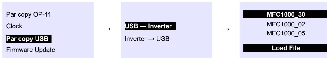
**Fig. 1.11.** Copying parameters settings: USB flash drive → Frequency converter
